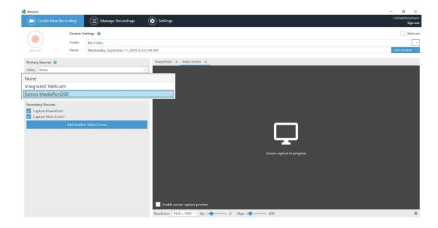
1.) First plug in the USB cable at the podium. It might take a minute to install some drivers. Once Panopto is opened up, click on the arrow by the video input to select the camera. The input should be labeled "AV Bridge" or "Extron Mediaport." Go ahead and select that input.
