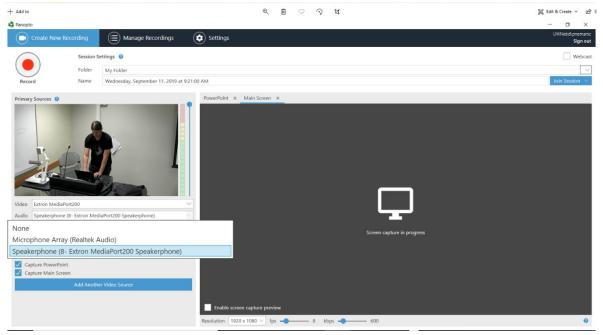
**2.)** Next, click on the arrow by the microphone and select the same **"AV Bridge"** input. To confirm audio is working, speak into the room microphone and levels should bounce on the audio meter.
